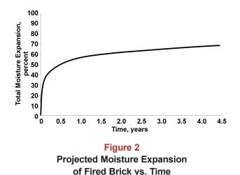
In brickwork, moisture expansion of the brick is somewhat offset by drying shrinkage of the mortar. As brick with larger face dimensions cover more wall area, the brickwork will experience more moisture expansion.
