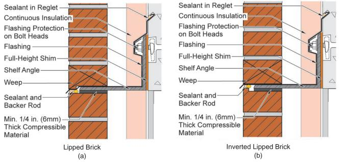
Figure 8 Alternate Expansion Joint Detail
