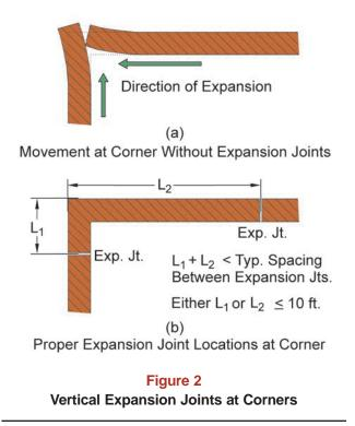
distances from a corner to first vertical expansion joint in each wall should not exceed the spacing of expansion joints in a straight wall, as shown in Figure 2b. For example, if the spacing between vertical expansion joints on a straight wall is 25 ft (7.6 m), then the spacing of expansion joints around a corner could be 10 ft (3.0 m) on one side of the corner and 15 ft (4.6 m) on the other side.
