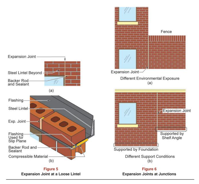
Locating the expansion joint adjacent to the window when using a loose-laid lintel will influence the dead weight of the masonry bearing on the lintel. The full height and thus weight of the masonry above the opening should be assumed to bear on the lintel instead of the triangular-shaped load typically assumed for loose-laid lintels. See *Technical Note* 31B for more information about steel lintel design.
