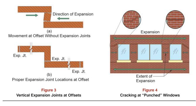
**Offsets and Setbacks.** As the ends of parallel walls expand, they tend to rotate the wall section that connects them, resulting in cracks, as shown in Figure 3a. Place expansion joints at the offset to allow the parallel walls to expand, as Figure 3b illustrates. Expansion joints placed at inside corners are less visible.
