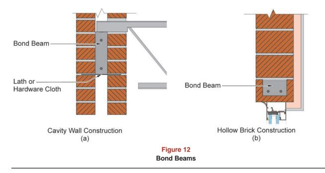
accommodate or distribute high stresses will also help control the effects of movement. Reinforcement can be placed in bed joints or in bond beams, as shown in Figure 12. Historic load-bearing structures were not constructed with expansion joints. However, these walls were constructed using multi-wythe brick construction, unlike typical structures built today.
