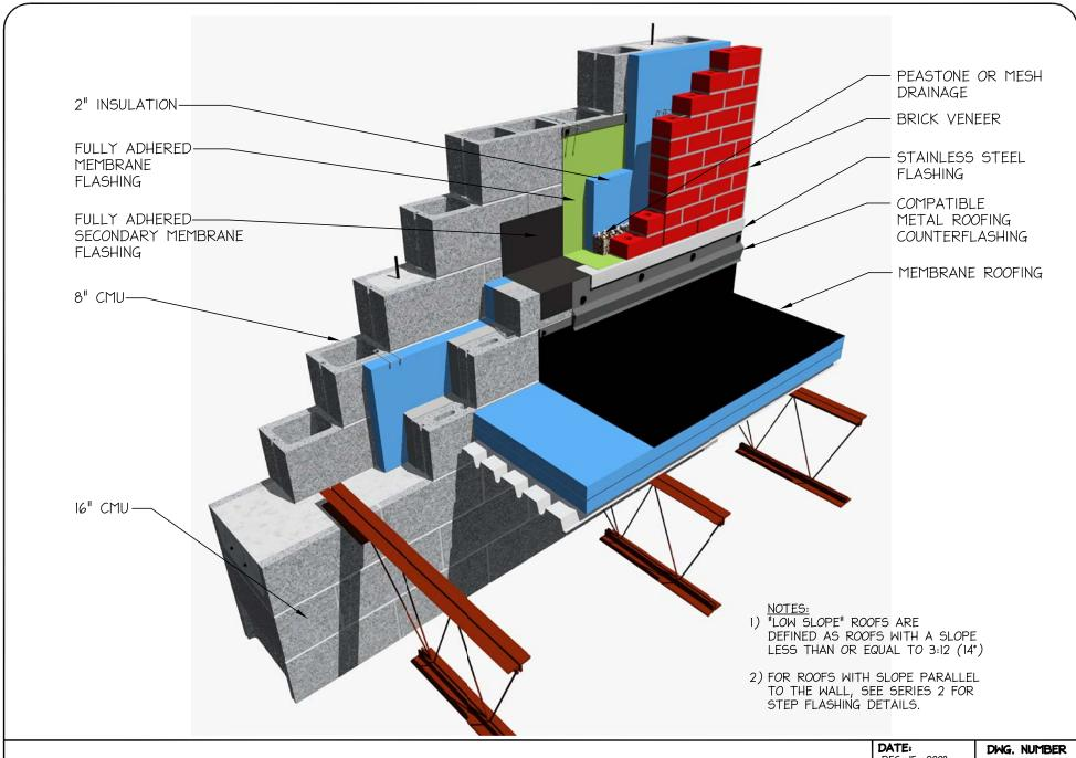
ISOMETRIC - HIGH CAVITY WALL FLASHING @ LOW SLOPE LOW ROOF
