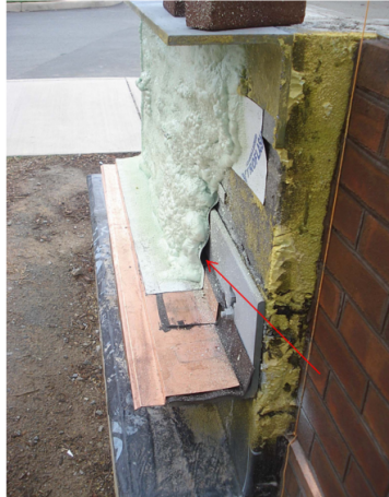
FIG. 5 Self adhered membrane adhesion loss observed on a building mock-up following the installation of SPF.
